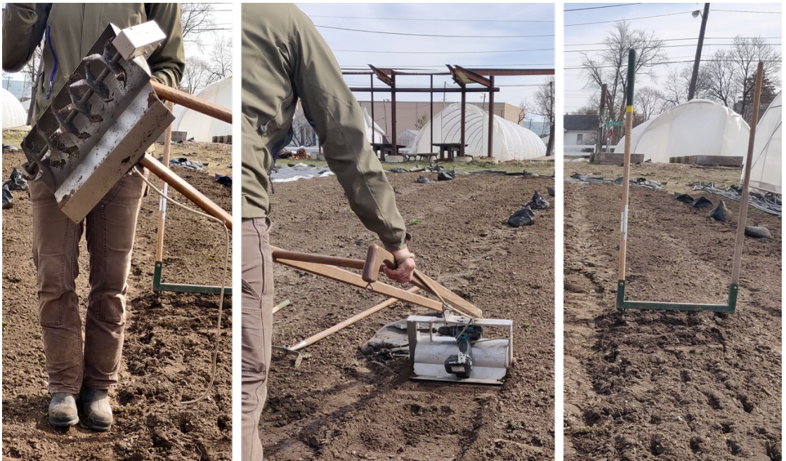
Figure 1: Tools at the City Farm. From left to right: The blades of the drill-driven tiller, the drill-tiller in use, and the broad fork, sunk into the earth
