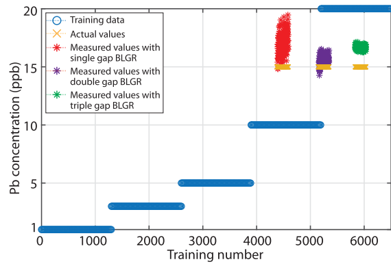
Fig. 8. Performance of the proposed machine learning algorithm in the presence of previously unobserved concentrations. Test results of a single-gap, double-gap, and triple-gap BLGR are spaced horizontally from left to right on the training datasets.
