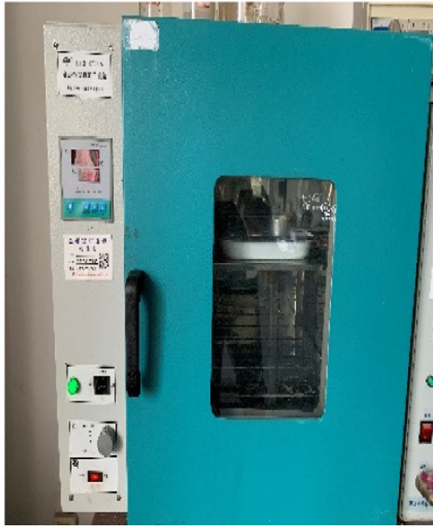
(b) Electric thermostat blast drying oven.
