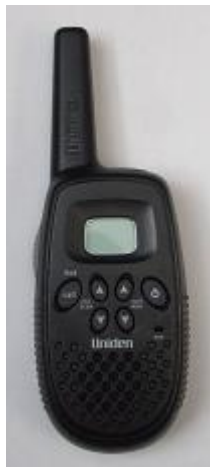
Fig. 22. Uniden GMR1636-2C radio, spun clockwise: (a) picture of the target, as seen from the antennas, (b) peak-pulse amplitude vs. angle for VV and VH polarizations; outer axis labels are in degrees; inner labels are in dBm.
