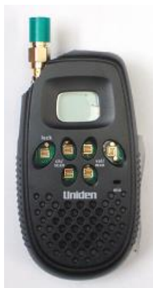
Fig. 23. Uniden GMR1636-2C with its antenna port terminated in 50\ \Omega , spun clockwise: (a) picture, as seen from the antennas, (b) peak-amplitude vs. angle for VV and VH; outer axis labels are in degrees; inner labels are in dBm.
