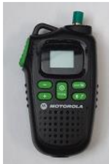
Fig. 10. Motorola MD200R radio with its antenna port terminated in 50 \Omega , rotated clockwise: (a) picture of the target, as seen from the antennas, (b) peak-amplitude vs. angle for VV and VH polarizations; outer axis labels are in degrees; inner labels are in dBm.
