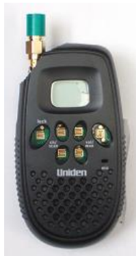
Fig. 12. Uniden GMR1636-2C with its antenna port terminated in 50\ \Omega , rotated clockwise: (a) picture, as seen from the antennas, (b) peak-amplitude vs. angle for VV and VH; outer axis labels are in degrees; inner labels are in dBm.
