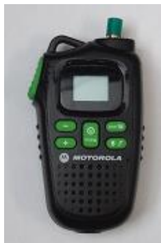
Fig. 21. Motorola MD200R radio with its antenna port terminated in 50\ \Omega , spun clockwise: (a) picture of the target, (b) peak-amplitude vs. angle for VV and VH polarizations; outer axis labels are in degrees; inner labels are in dBm.
