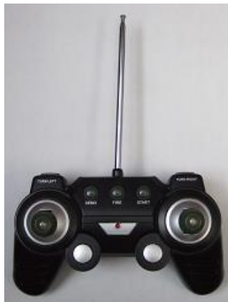
Fig. 13. 27-MHz remote-controlled toy tank transmitter, rotated clockwise: (a) picture of the target, (b) peak-pulse amplitude vs. angle for VV and VH polarizations; outer axis labels are in degrees; inner labels are in dBm.
