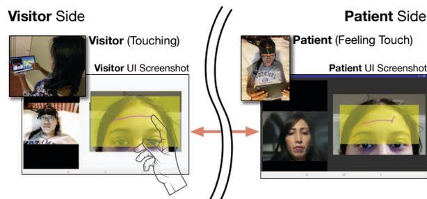
Figure 1: Diagram of our tactile telepresence system prototype, with examples of real users and the visitor/patient user interfaces.
