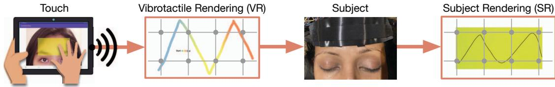
Figure 2: The overall tactile recognition evaluation process, comprising two steps: the input and vibrotactile rendering of a touch pattern (VR), and the subject-drawn rendering of the perceived pattern (SR).
