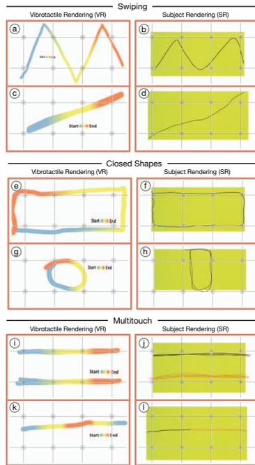
Figure 3: Sample actual and subject-interpreted patterns representing (a)–(d) continuous swiping motions, (e)–(h) closed shape patterns, and (i)–(l) multiple fingers moving simultaneously (multitouch).
