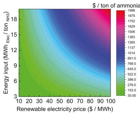
**Figure 7.** Input cost of green ammonia synthesis as a function of renewable electricity price and the energy input. The input cost of natural gas for making a ton of ammonia in the Haber–Bosch process is relatively constant and is about \$150 (~35 314.7 ft<sup>3</sup> of natural gas). The hatched area is where renewable ammonia synthesis will have comparable or lower input cost than the conventional process.
