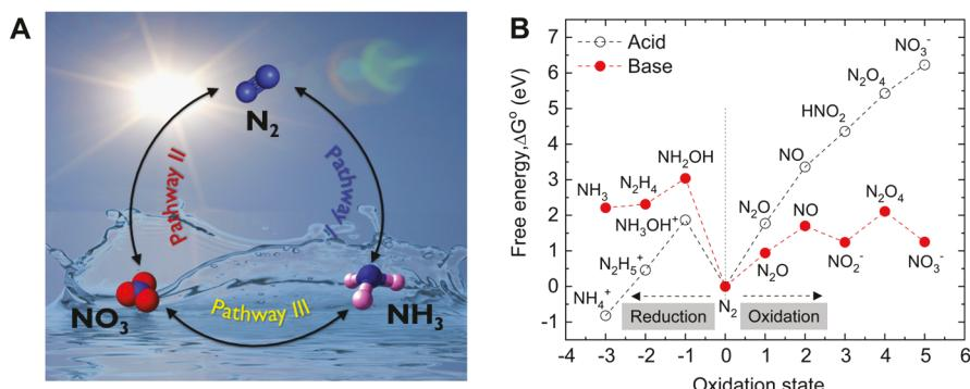
**Figure 1.** (A) Various routes for interconversion of nitrogen and nitrogen-containing compounds to enable a circular nitrogen economy. (B) Free energy diagram for nitrogen oxidation and reduction states in acidic and basic solutions. Data from ref 28.
