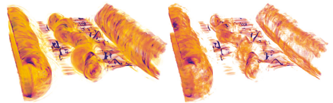
Fig. 10: Volume rendering of the magnetic reconnection event dataset at full resolution (left, 512 MB) and AMM (right, 9.86 MB) are shown, highlighting the flexibility of AMM to handle different types of (dense vs. sparse) datasets and still highlight important features therein.
