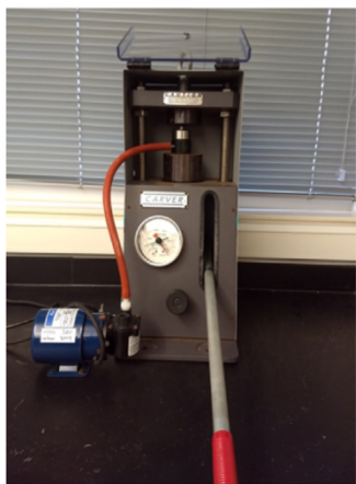
Fig. 2. The hydraulic press used for pelletization along with the die assembly in place. A detachable vacuum pump was attached for simultaneous pumping out of air for more compact pellet making.
