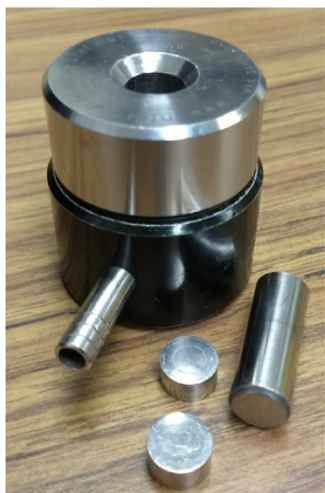
Fig. 1. The die assembly used for pelletization using a hydraulic press. The black bottom acts as an assembly holder and can be connected to a vacuum pump while pressing. The two circular discs are the dies between which the powder is placed and the cylindrical rod helps in applying pressure uniformly during pressing.
