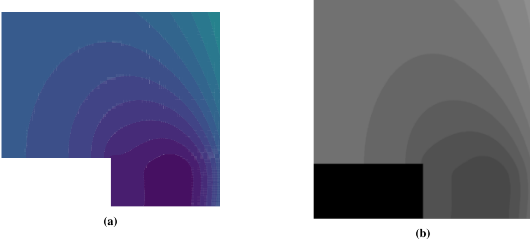
Fig. 3 HF pressure output from a flow over a backward facing step: (a) Y_{HF} contour vector output, and (b) P_{HF} contour pixel output.
