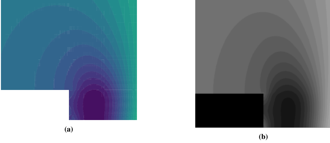
Fig. 2 LF pressure output from a flow over a backward facing step: (a) Y_{LF} contour vector output, and (b) P_{LF} contour pixel output.
