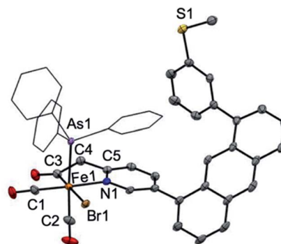
Fig. 1 ORTEP representation (30% thermal ellipsoids) for [(Anth·C H2 NS off )Fe(CO) 2 (Br)(AsPh 3 )]. Hydrogen atoms are omitted for clarity and the phenyl groups of AsPh 3 are depicted as wireframes. Selected bond distances (Å) and bond angles (°): Fe1–C3 = 1.942(3), Fe1–N1 = 2.036(2), Fe1–As1 = 2.4050(5), C3–Fe1–N1 = 83.55(11), C3–Fe1–As1 = 91.76(11), N1–Fe1–As1 = 88.97(6).
