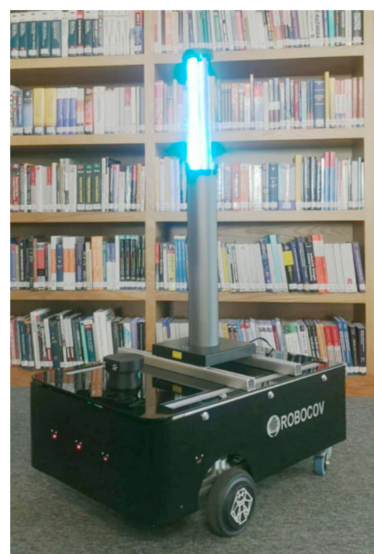
Figure 27. UV module operating in the library.
