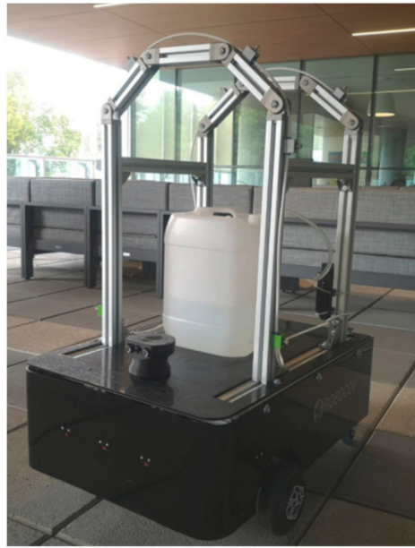
Figure 28. Operating atomizer disinfection module working on open spaces.
