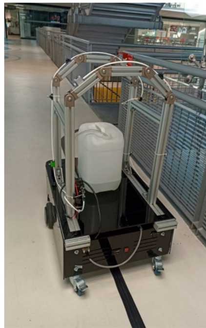
Figure 2. Following a line for repetitive tasks.
