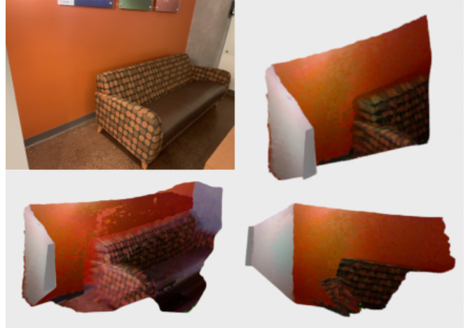
Fig. 1. Registration result of point clouds from 93 frames with our proposed framework using 3D points, 3D lines and 3D planes. The scene contains texture-poor areas, which are difficult for methods that rely on 2D features derived from color images.
