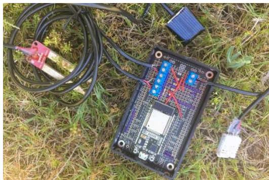
Figure 1. Agrivoltaic School Garden Monitoring Device
