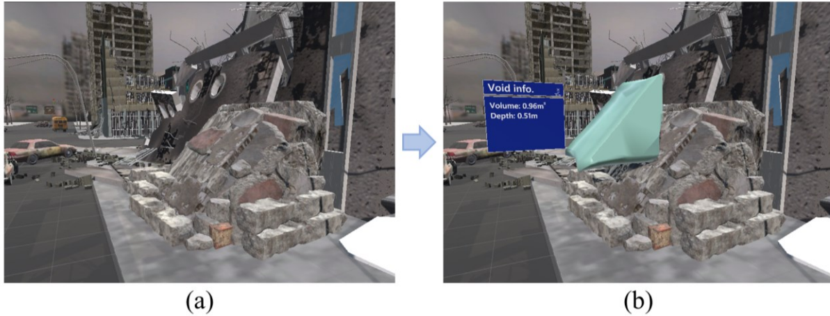
Fig. 10. Interface of the AR system prototype: (a) disaster rubbles; and (b) disaster rubbles with void information overlaid
