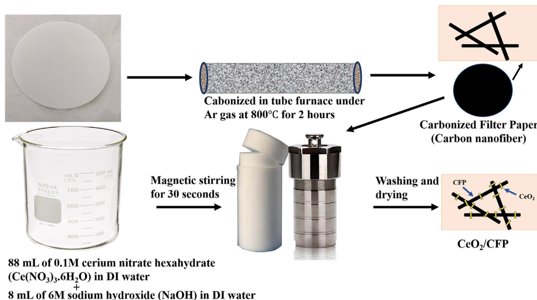
Fig. 2. Schematic illustration of the preparation of the CFP and \text{CeO}_2/\text{CFP} interlayer.
