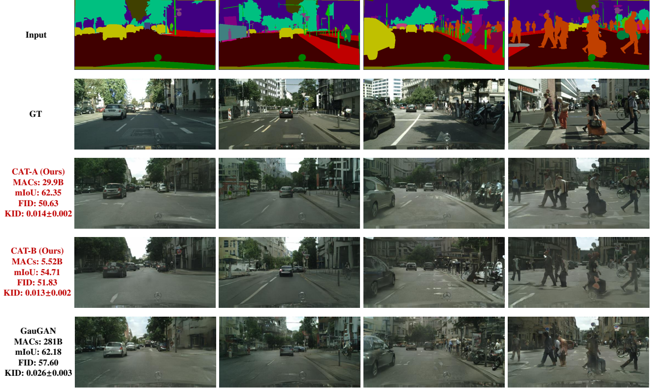
Figure 4: Qualitative results on Cityscapes dataset. Images generated by our compressed model (CAT-A, third row) have higher mIoU and lower FID than the original GauGAN model (fifth row), even with much reduced computational cost. For our CAT-B model (fourth row, 50.9\times compressed than GauGAN), although it has lower mIoU, the CAT-B model can synthesize higher fidelity images (lower FID) than GauGAN.
