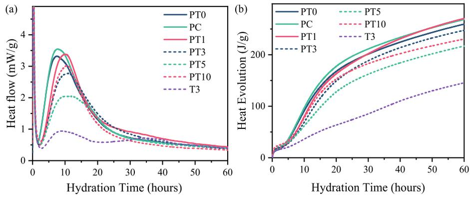
Fig. 5. Effect of the proposed pre-hydration process on the hydration of the cement: (a) thermal power; (b) Accumulated hydration heat.
