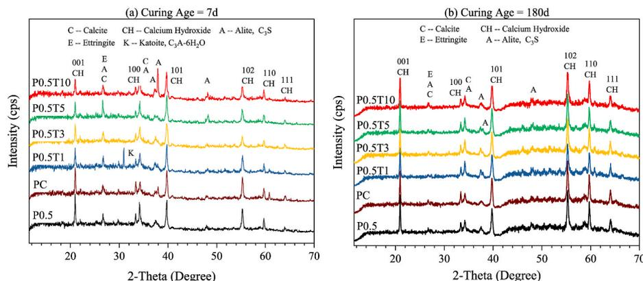
Fig. 7. XRD patterns of produced pastes after sealed curing for (a) 7d; (b) 180d.
