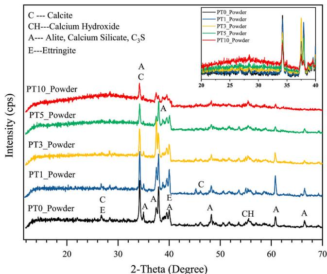
Fig. 2. XRD patterns of produced filtered powders after the pre-hydration process.
