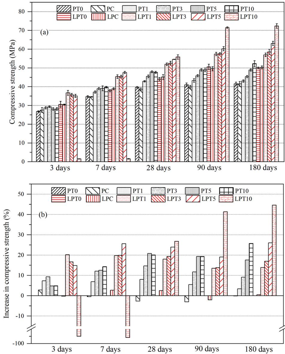
Fig. 6. Improvement on the compressive strengths achieved by the proposed method: (a) the compressive strength; (b) the increase % compared to the compressive strength of the control groups PT0 or LPT0.
