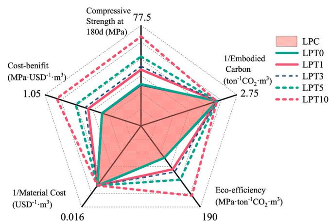
**Fig. 13.** Five-dimensional assessment considering mechanical properties, embodied carbon, eco-efficiency, materials cost, and the cost benefit (strength per unit cost) of mortars with w/b of 0.45. The calculated embodied carbon and materials cost are based on 1 m<sup>3</sup> of mortars.
