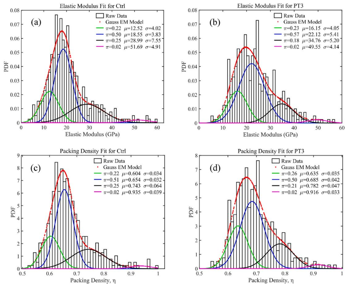
Fig. 11. Deconvolution results of the elastic modulus ( $E$ ) and packing density ( $\eta$ ) of nanoindentation: (a) The elastic modulus for Ctrl; (b) The elastic modulus for PT3; (c) The packing density for Ctrl; and (d) the packing density for PT3.
