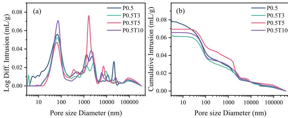
Fig. 9. Pore size distribution for the mortars mixed with prehydration process: (a) Log differential intrusion; (b) Cumulative intrusion.
