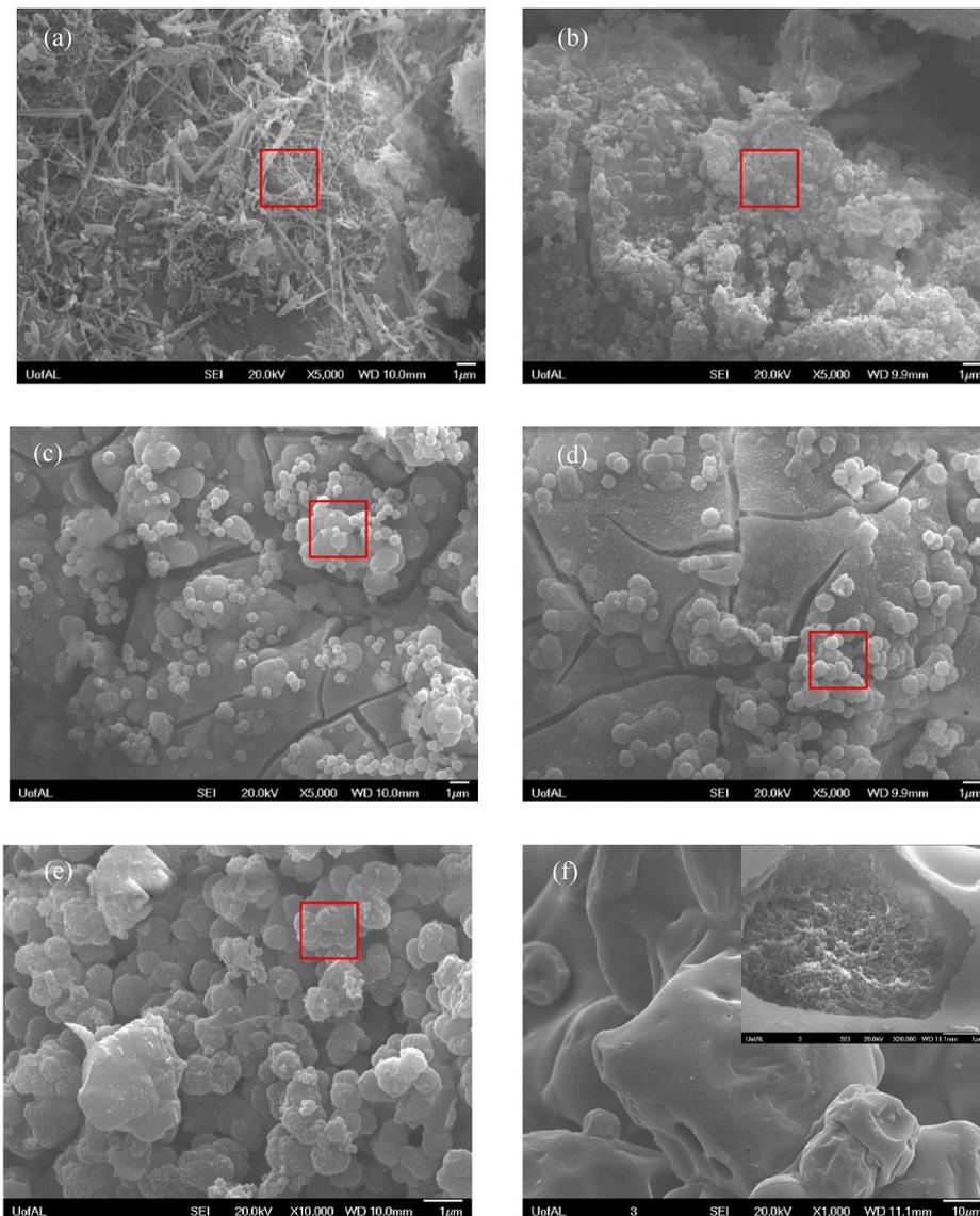
**Fig. 1.** SEM images of filtered particles produced by pre-hydration with TA: (a) PT0\_Powder; (b) PT1\_Powder; (c) PT3\_Powder; (d) PT5\_Powder; (e) PT10\_Powder; (f) Pure TA powder.
