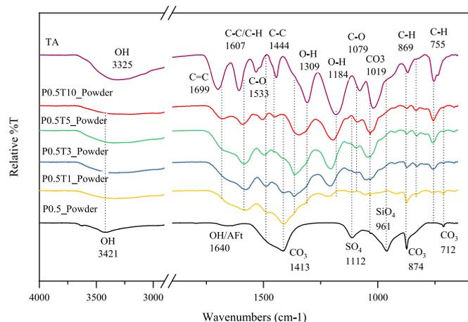
Fig. 3. FTIR patterns of produced filtered powders by the pre-hydration process.
