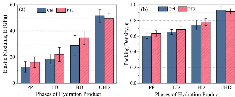
Fig. 12. Comparison of indentation properties of four different phases of hydrates for Ctrl and PT3: (a) Elastic modulus; and (b) Packing density.
