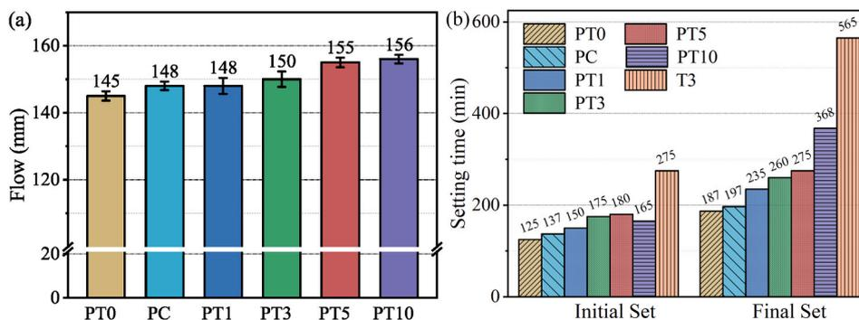
Fig. 4. Properties of the fresh mortars mixed with pre-hydration process: (a) flowability (mm) and (b) setting time.
