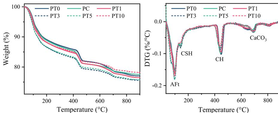
Fig. 8. TGA curves of the produced pastes after 7d sealed curing with the pre-hydration process.
