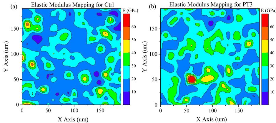
Fig. 10. Contour mapping of elastic modulus obtained from grid of nanoindentation: (a) Control cement pastes (Ctrl); and (b) Cement paste made by premixing with 0.3% TA (PT3).
