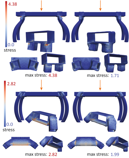
Fig. 27. Bench stress for twisted and bended set of legs
