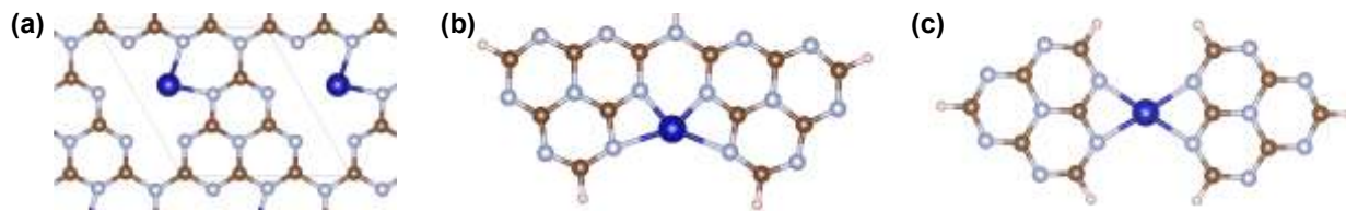
Figure 3. Structures of single \text{Co}^{2+} sites coordinated with N atoms in \text{C}_3\text{N}_4 : (a) \text{Co-N}_2 , (b) \text{Co-N}_4 , and (c) \text{Co-N}_{2+2} at edge sites. Color scheme: Co (blue), N (silver), C (gold), H (light brown).
