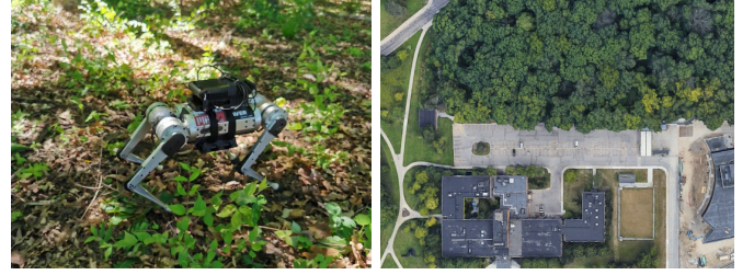
Fig. 1: MIT Mini-Cheetah robot with a customized sensor suite and satellite map of the data collection environment for this work. The Mini-Cheetah robot is equipped with an Intel RealSense depth camera, an Inertial Measurement Unit (IMU), and an Nvidia Jetson Xavier computing device for data recording. Motion and task planning for legged robots in unstructured environments involve explicitly modeling the terrain traversability and solving a sequential decision-making problem to find the “optimal” behavior. For unknown environments, terrain traversability modeling using noisy measurements is itself a challenging problem due to the lack of a priori knowledge of the surrounding terrain, the variability of terrain conditions, and the robot-specific characteristic of traversability.
