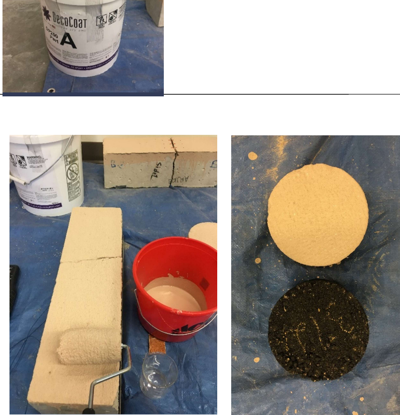
Figure 14. Application of the coating using a roller brush onto the concrete and asphalt surfaces.
