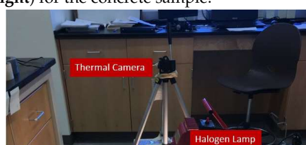
Figure 9. Experimental setups of controlled heating ( left ), airflow heating ( center ) and humid heating ( right ) for the concrete sample.
