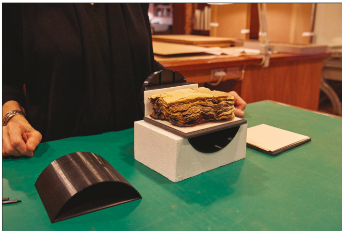
FIGURE 2. The M.910 manuscript is prepared for placement in the scanner. Foam and support boards ensure a firm but reasonable fit against the manuscript.
