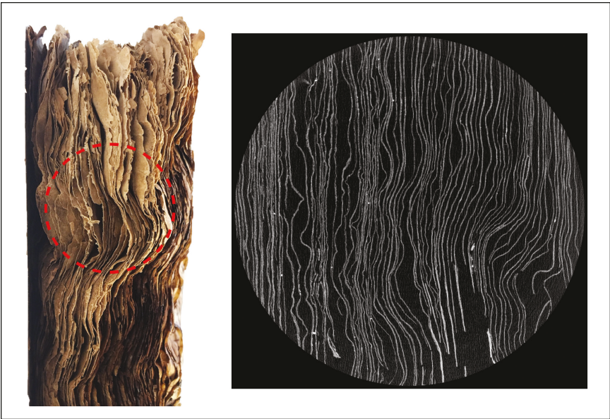
FIGURE 5. By zooming in on the core of the manuscript (left, image not to scale), we were able to achieve a sixteen-micron resolution scan (right). One can see the distorted and torn individual leaves of the manuscript in the slice image.
