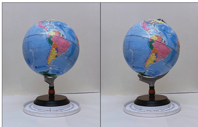
Fig. 4. A globe mounted on a turntable. The globe rotates 30^\circ counterclockwise and the turntable 30^\circ clockwise from its starting position (left) to produce the right frame of a stop-motion animation.
