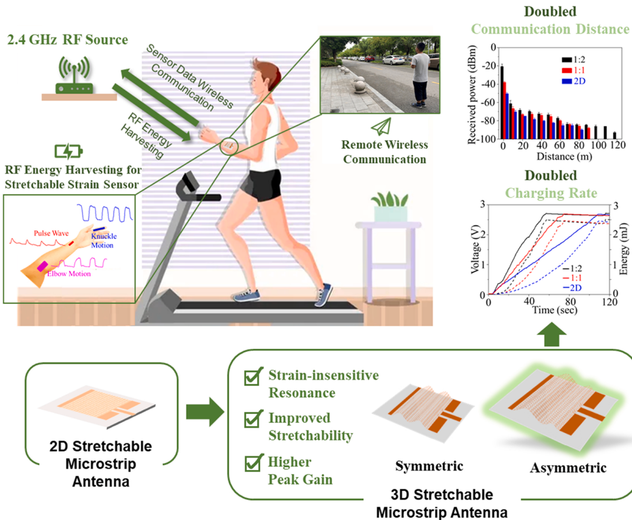
Fig. 1. Design concepts of the standalone stretchable RF systems based on asymmetric 3D microstrip antennas with excellent on-body wireless communication and energy harvesting.
