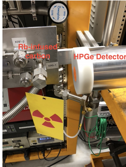
Figure 2. Location of the HPGe detector for the source activity measurement. The detector was placed at a known distance from the ^{83}\text{Rb} source, which was inside the steel VCR container shown in the picture.
