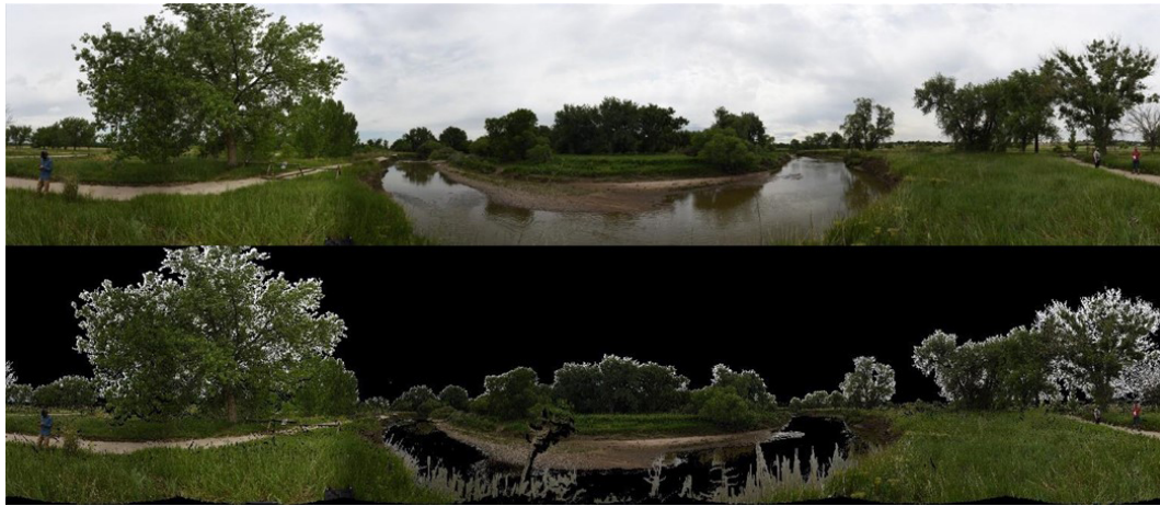
Figure 3. The top shows the terrestrial laser scanner photograph from a scan location, whereas the bottom shows the associated point cloud at the Cache la Poudre River site. Courtesy of UNAVCO.
