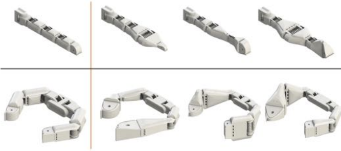
Fig. 5. Morphology design space. The initial morphology of the single finger and the two-finger gripper designs are shown on the left. We randomly sample different parameters for each configuration and show the deformed morphology on the right.
