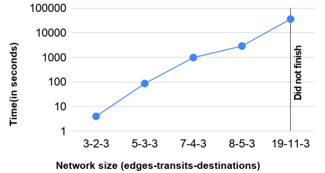
Figure 5: Growth of solution time for the optimization model with network size. The optimization model is impractical and unscalable for a real system deployment.
