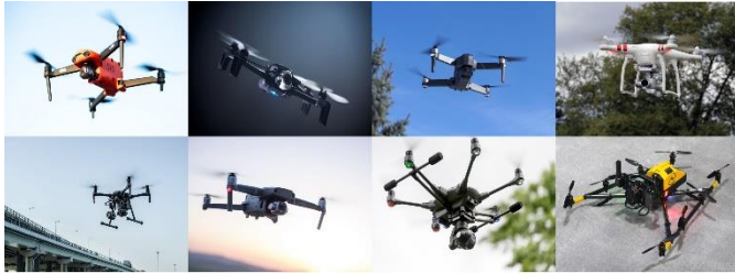
Figure 1. Drones that are Included in the Review. From the Top Left Autel Evo II, Parrot Anafi, Ruko F11 Pro 4K, DJI Phantom 3, DJI Matrice 200, DJI Mavic 2 Pro, Yuneec Typhoon H, Intel Falcon 8+
