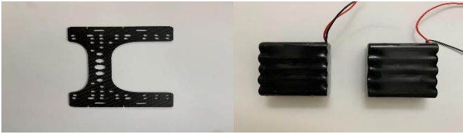
Figure 3. The Carbon Fiber Frame and the Battery Packs
