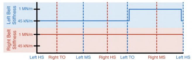
Fig. 3. Timing of unilateral stiffness perturbation within one gait cycle. Note that: HS, MS, and TO stand for heel strike, mid-stance, and toe-off respectively. The stiffness is adjusted to rigid during the swing phase, when the leg is not touching the treadmill, to avoid oscillations of the belt after the leg pushes off.
