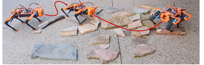
Fig. 1. Legged locomotion over complex terrain. Example of a trajectory taken by the OpenQuadruped robot using sim-to-real transfer of a linear policy on difficult terrain.
