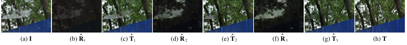
Figure 3. The gradual refinement of reflection removal results after each iteration. The input image \mathbf{I} is taken in front of a window glass.
