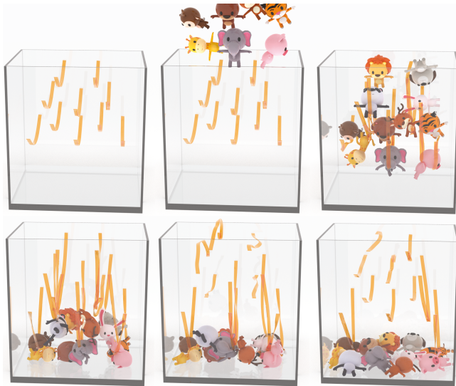
Fig. 16. “Animal crossing”. A pack of soft animal characters fall and hit several rubber straps. There are 21 deformable objects in this example consisting of 293K elements. The falling animals induce interesting deformation effects: a couple of straps get entangled with the animals and are pulled to the floor. The runtime simulation FPS is between 13.4 to 46.3.
