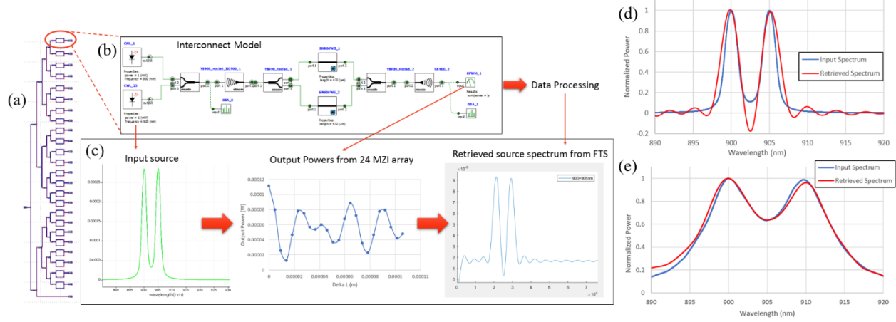
Fig. 2. (a) SHFTS design floor plan. (b) Compact Interconnect model for each MZI. (c) Overall FTS operation procedure. Input and retrieved spectrum from FTS with various input sources: (d) Peaks are separated by 5 nm ( \lambda=900 nm and 905 nm). (e) Peaks are separated by 10 nm ( \lambda=900 nm and 910 nm).
