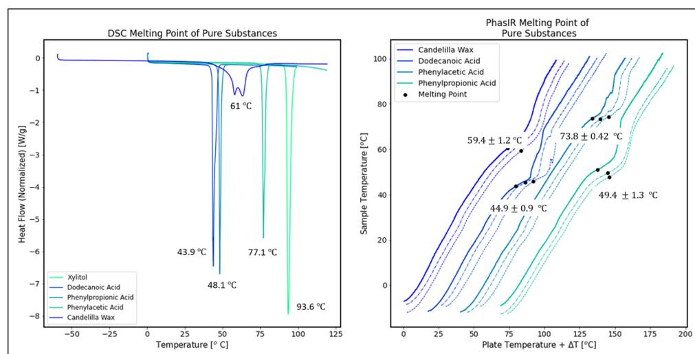
**Figure 9** Results of melting point determination for pure substance using DSC (left) and PhasIR (right).
