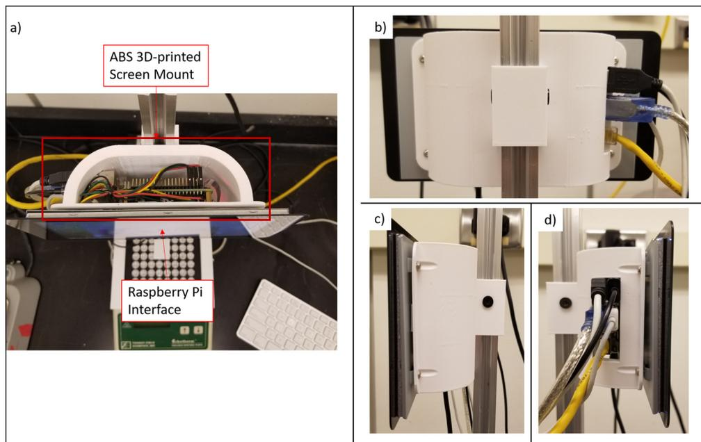
**Figure 6** Raspberry Pi control system. **a)** Inside view of screen and Raspberry Pi 3B+ mount. **b), c), d)** Rear and side views of mount.
