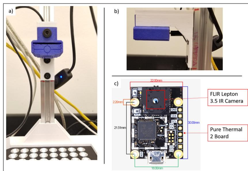
**Figure 3** Lepton 3.5 and PureThermal 2. **a)** Front view of mounted camera and board. **b)** Side view of mounted camera and board. **c)** Schematic of Lepton 3.5 attached to PureThermal 2 board.
