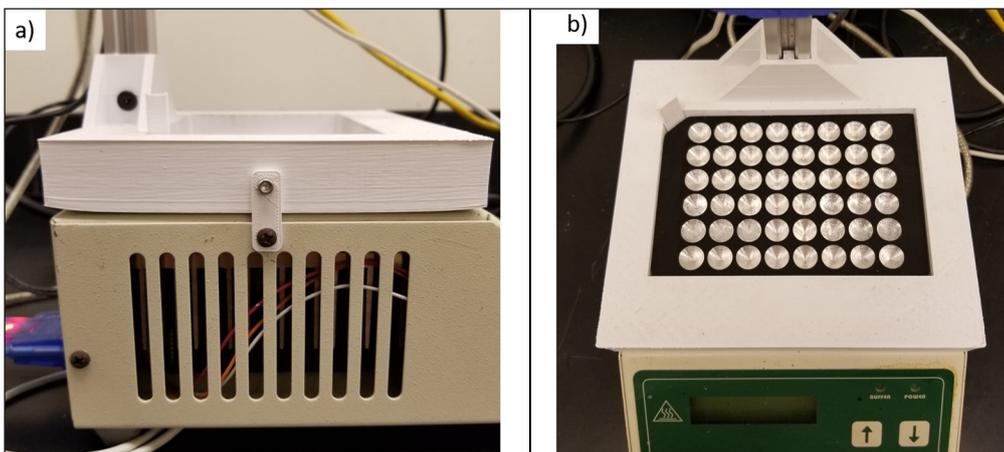
**Figure 5** Enclosure and Conical Well Plate. **a)** Side view of enclosure mounted on to the Echotherm IC25 via a set of screws. **b)** Top view of the Echotherm IC25 and enclosure with conical-well 48 well plate inside.
