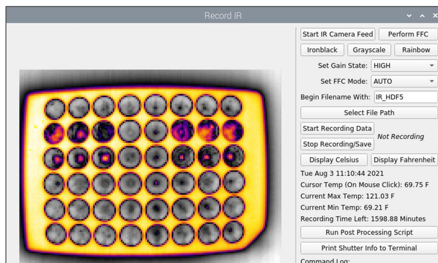
**Figure 4** Example window of the image capture software *purethermal1-uv-capture*. A real-time image of the system is displayed on the left, while the right panel allows the user to interact with the camera, start the data collection and save the results into an .HDF5 file.
