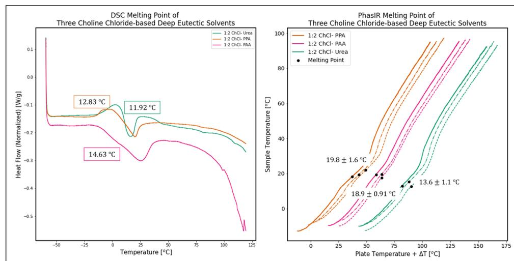
**Figure 11** Results of melting point determination for three Choline Chloride-based Deep Eutectic Solvents using DSC (left) and PhasIR (right).
