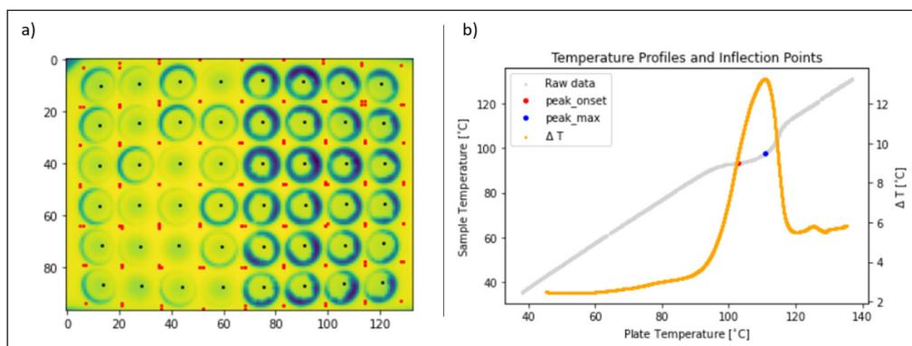
**Figure 8 a)** Example 48-well plate with centroid and plate temperature identification obtained through the PhasIR Image Analysis module. The black marker identifies the centroid of the well, whereas the red marked are used as the reference plate temperature for each well. **b)** Example result temperature curve for a single sample (Dodecanoic Acid). The phase transition temperature is the determined automatically as the onset of the peak in the curve (yellow).
