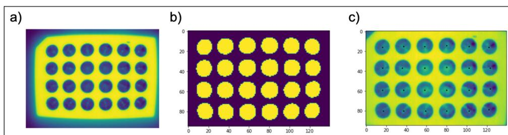
**Figure 7** Example output of PhasIR image analysis module. **a)** Raw frame from .HDF5 video from Lepton 3.5 IR camera. **b)** Output of automatic object (well) recognition. **c)** Result of automatic centroid (black markers) fitting of each well in the plate.
