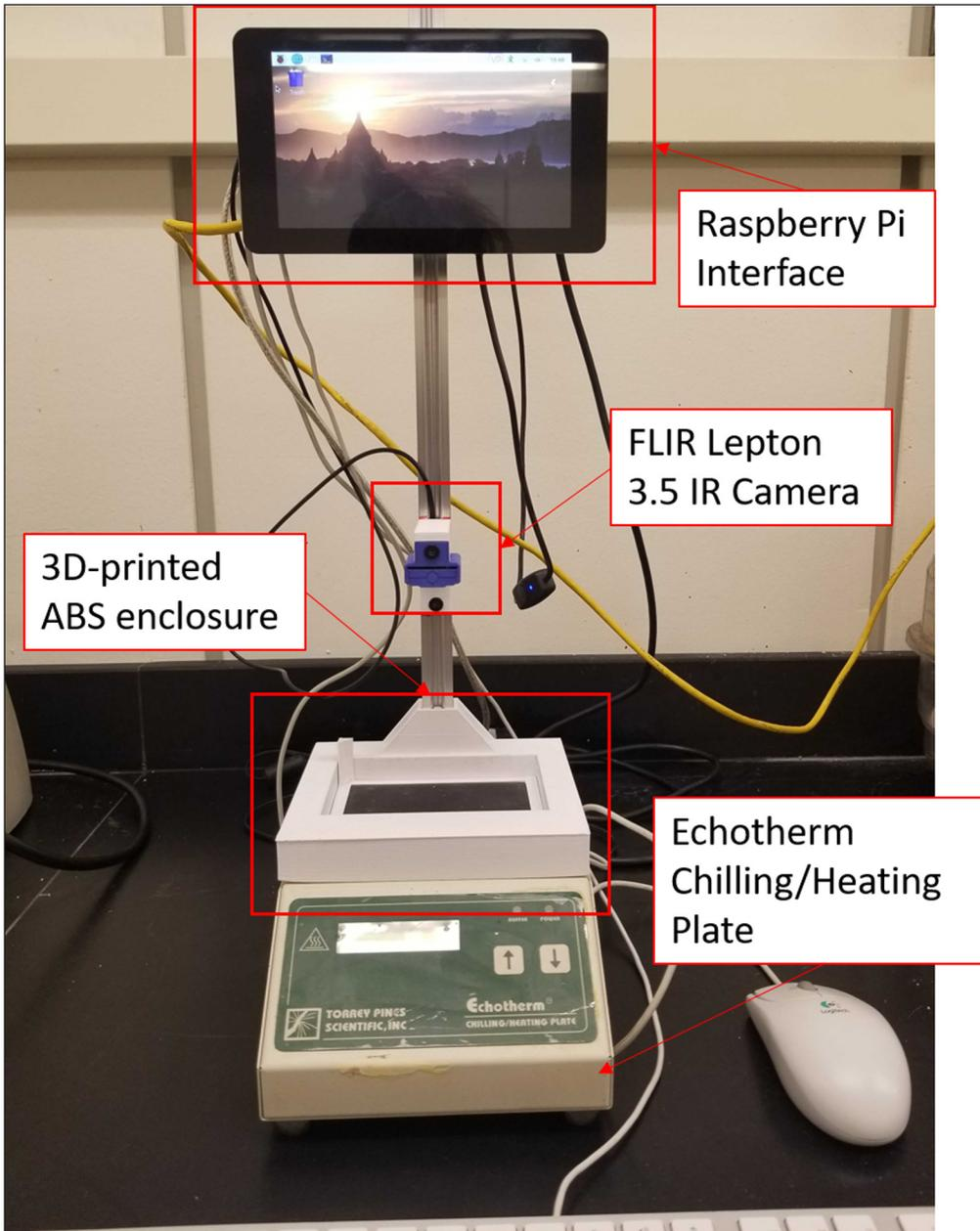
**Figure 1** PhasIR Hardware System. This is composed of a Raspberry Pi Interface, an IR Camera, a 3D printed plate enclosure and a Peltier plate.
