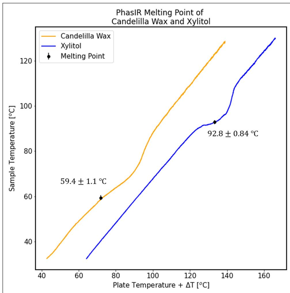
**Figure 10** Results of melting point determination for candelia wax and xylitol on a 48-well plate.
