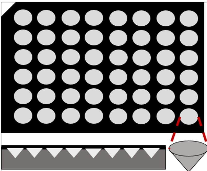
**Figure 2** Schematics of the aluminum well plate design. The top of the plate is coated in black paint to obtain an emissivity of one. The wells have a conical shape to ensure consistent sample location throughout the phase transition process.
