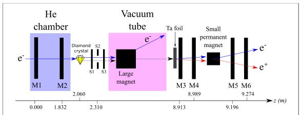
**Figure 1.** A schematic representation of the experimental setup during the diamond experiment in the H4 beam line in the SPS North Area at CERN. The symbols 'Sj', with j=1,2,3, denote the scintillators and the symbols 'Mi', with  $i=1,\ldots,6$ , denote 'Mimosa-26' position sensitive detectors with a resolution of 3.5  $\mu$ m.
