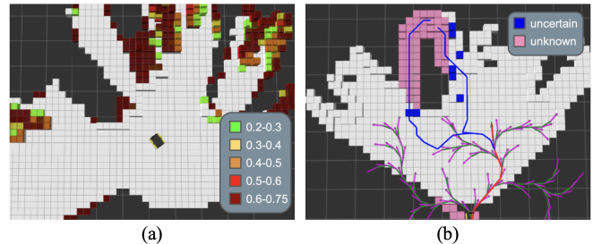
Fig. 1. The NBV planner in action in a simulated environment. (a): Example Octomap map. White cells: ground and obstacles cells with occupancy probability \geq 0.75 ; colored cells: uncertain occupancy probability, but potentially safe. (b): NBV planner first stage. Candidate NBV poses are in purple, the best one is in red (along with the first common trajectory segment) and the two path hypotheses are in blue.
