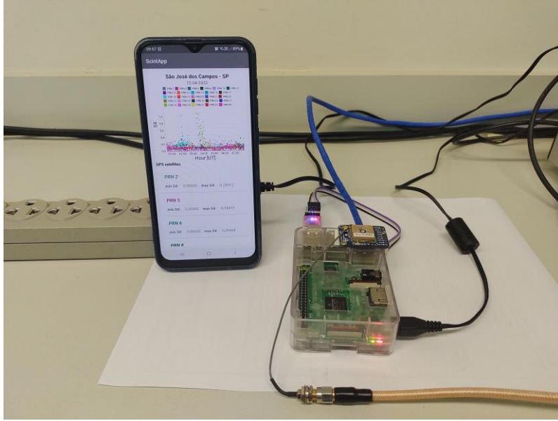
Figure 9: Android mobile device running ScintApp next to the IoT based scintillation monitor prototype Ionik2 installed at Instituto Tecnológico de Aeronáutica in São José dos Campos (23.209°S, 45.874°W).
