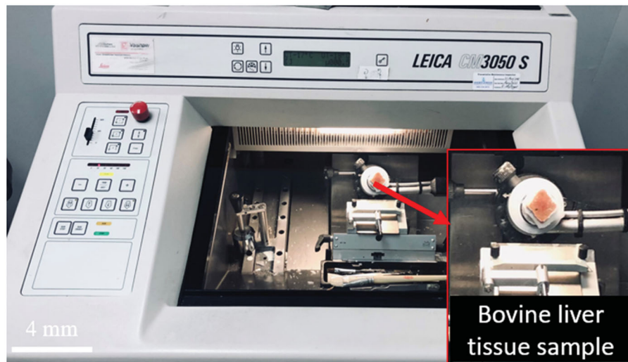
Figure 3. The cryostat machine for sectioning the bovine liver tissue samples with a thickness of 0.5\ \mu\text{m} .
