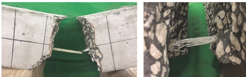
Fig. 7—Typical GFRP bar tensile rupture failure at midspan.
