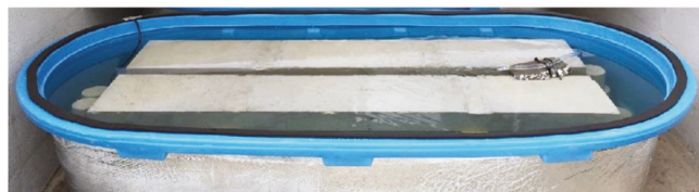
Fig. 2—Accelerated-aging setup (seawater at 60°C [140°F]).
