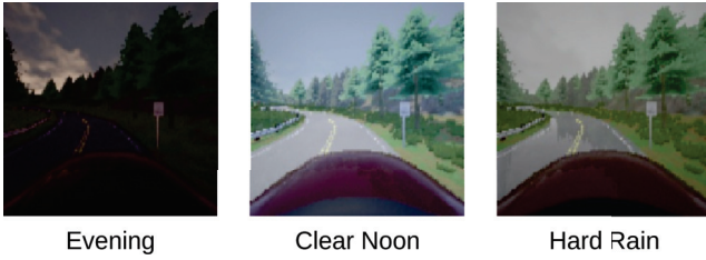
Figure 3: Experiment of the driving task in CARLA simulator. Examples of the driver view (observation states) under three different weather conditions: evening, clear noon and hard rain from left to right.
