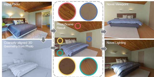
Figure 1. Given an input photo and a coarsely aligned 3D scene model, PhotoScene automatically infers high-quality spatially-varying procedural materials and scene illumination to closely match scene appearance. The reconstructed materials are resolution-independent (see zoom insets) and ascribed to the full 3D geometry, to create a high-quality photorealistic digital twin that can be rendered under novel views and lighting.
