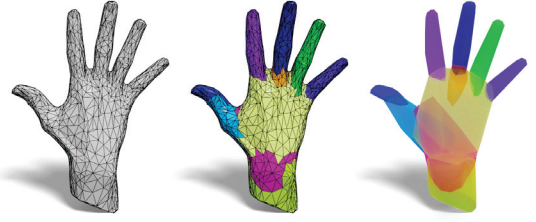
Fig. 6. An example of triangle-grouping-based methods (from HACD). From left to right: (a) Input triangle mesh. (b) Grouping results of the triangle faces, where each color indicates a component. There are zig-zag boundaries between different components. (c) Corresponding convex hulls of each component, and they intersect with each other.
