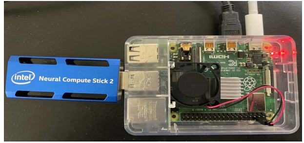
Fig. 2: Intel NCS2 with Raspberry Pi 4B as host board.
