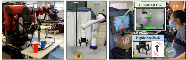
Fig. 1: Tele-nursing assistance tasks may involve freeform, dexterous manipulation (e.g., inserting a straw to the beverage container). Haptic and AR visual cues can be leveraged to communicate task-critical information.
