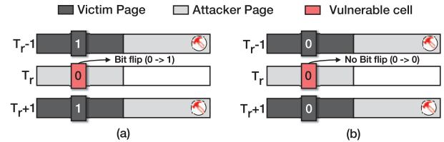
Fig. 1: Data dependency for inducing a rowhammer fault. Here, based on the presence of bit flip in the attacker-controlled vulnerable bit in the target row ( T_r ), data from adjacent row from victim program can be inferred.
