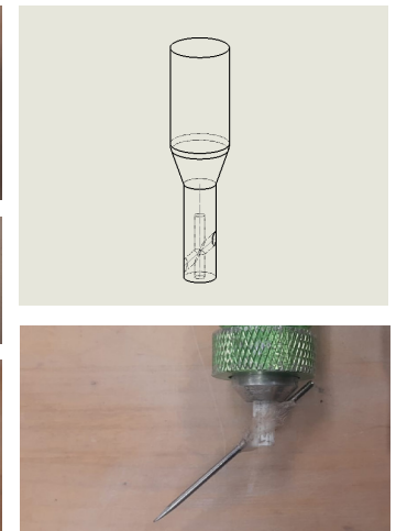
Figure 26. Adapted Hyrel printer head for angled grooving.
