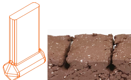
Figure 27. Round-tipped grooving design
