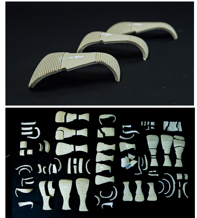
Figure 29. Ceramic samples used to chart the relationship between the grooving and the morphing.
