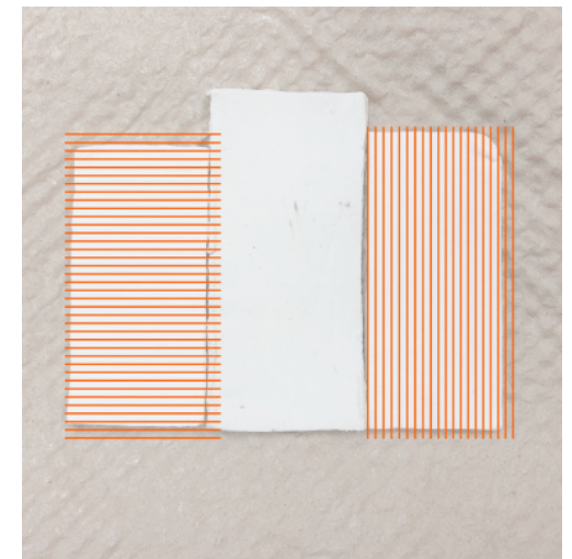
Figure 21. Left. Bi-layer layer testing of printing orientation
