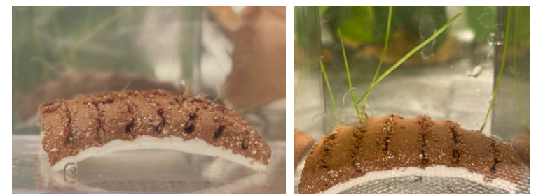
Figure 28. Round-tipped grooving design showing seeds growing on the tile.
