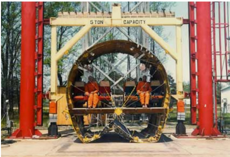
Fig. 1. Drop of a section of a Boeing 707 aircraft to the ground from a height of 55 ft and the visible damage.
