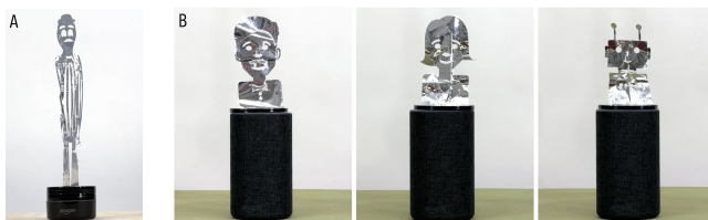
Figure 17: A) We instrumented an Amazon Echo dot with a 40cm pop-up butler, which could activate upon speaking a wake word. B) Users could also personalize their smart speaker agents with inexpensive (<$1) and swap-able avatar pucks, which rest on top of the speaker.
