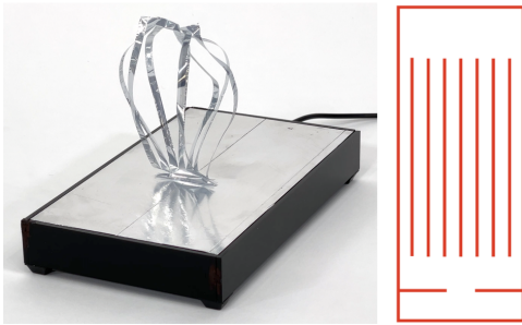
Figure 8: Multiple parallel slit cuts create ribbon-like features which repulse one another to form a sphere-like structure upon application of electrostatic charge.
