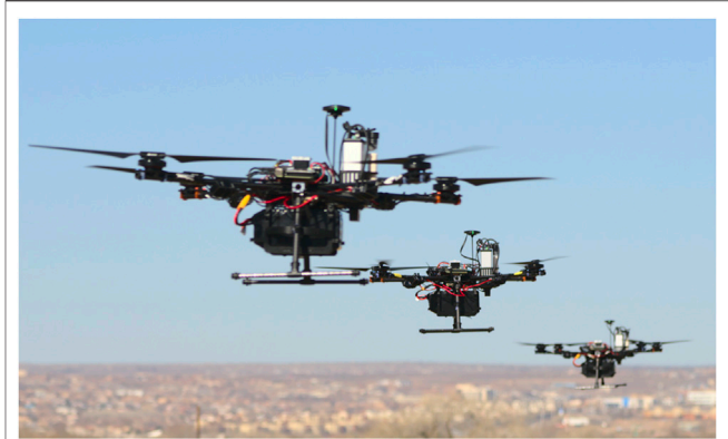
FIGURE 1 | Flocking Dragonfly UAVs in formation. The flocking Dragonfly UAVs are used to survey volcanic CO 2 plumes.
